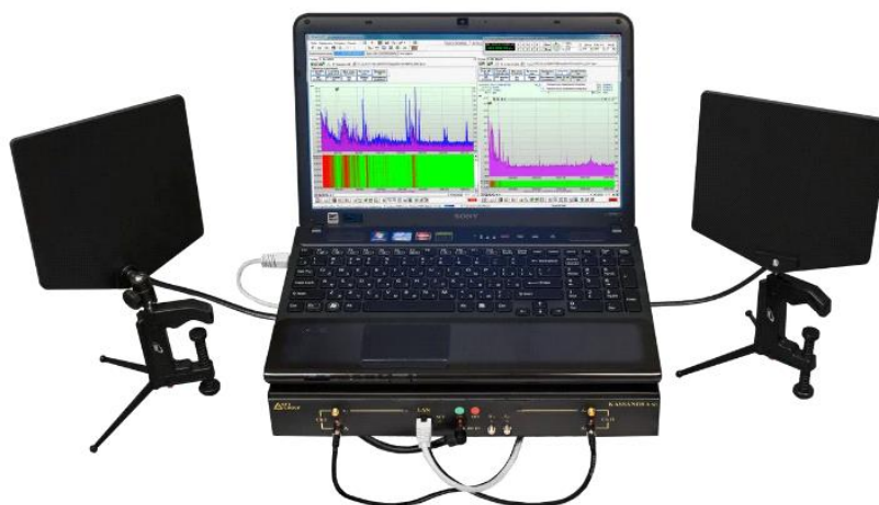
Fig.1. Appearance of search ASE Kassandra with ST 'RadioInspectorSoft'™
