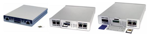
AVTOR's IP encryption complex is a totality set of tools, which is necessary and sufficient for construction of a Virtual Private Network (VPN) through any IPv4-networks. The information is transmitted over IPv4-networks in tunnel mode when the original IP-packets are encrypted and
