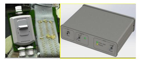
The system of protection intended to protect radio aviation channels against eavesdropping. The system consists of device for protecting negotiation - flight operator, pilot and software for generating and managing of key information and provides cryptographic protection of information transmitted by analogue radio channels of the ultra-short waves and short waves range.
