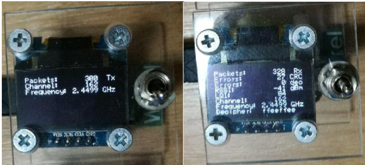
Fig. 6. Hardware receiver and transmitter on Pololu Wixel model with OLED
